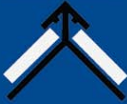
External capped corner
